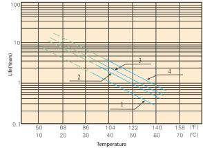
1----- For FM series 2----- For FML series 3----- For FMH series 4----- For GFM series
